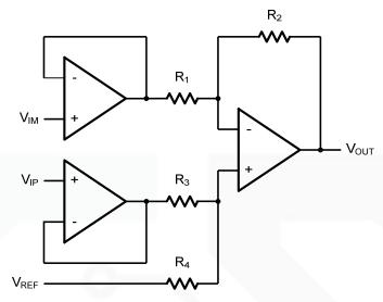
Figure 6. Instrument Amplifier
