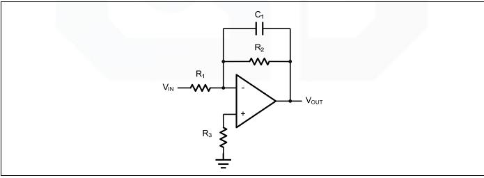
Figure 5. Low Pass Active Filter
