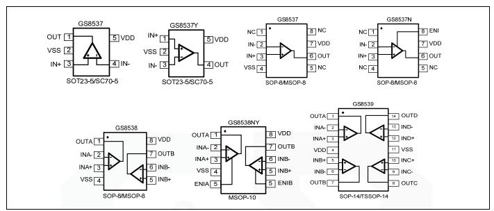
Figure 1. Pin Assignment Diagram
