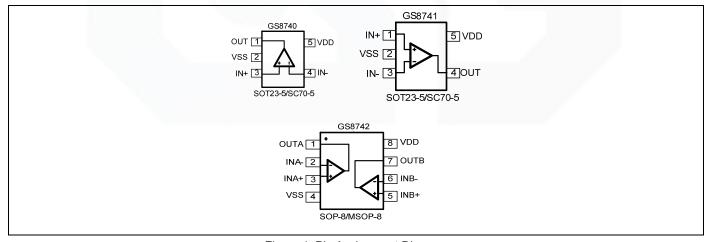
Figure 1. Pin Assignment Diagram
