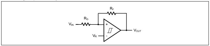
Figure 2. Non-Inverting Comparator with Hysteresis
