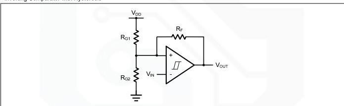
Figure 3. Inverting Comparator with Hysteresis
