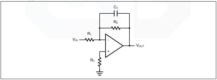
Figure 5. Low Pass Active Filter
