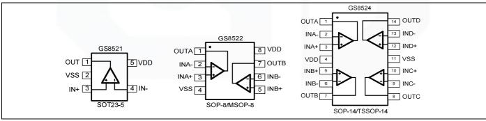
Figure 1. Pin Assignment Diagram
