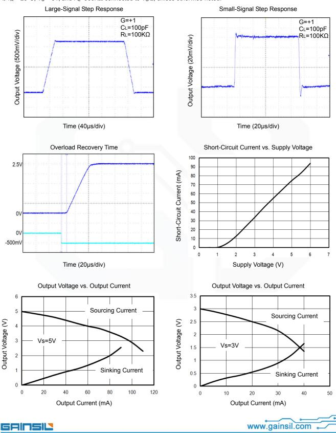
At T<sub>A</sub>=+25°C, V<sub>S</sub>=+5V, and R<sub>L</sub>=500K $\Omega$  connected to V<sub>S</sub>/2, unless otherwise noted.
