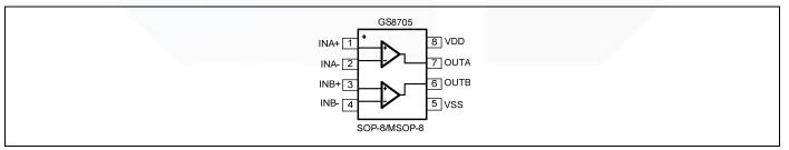
Figure 1. Pin Assignment Diagram
