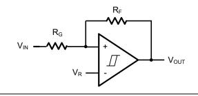
Figure 3. Non-Inverting Comparator with Hysteresis
