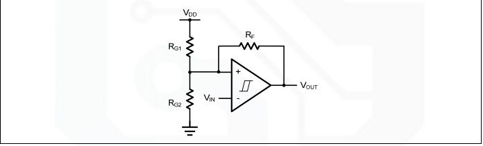
Figure 4. Inverting Comparator with Hysteresis
