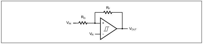
Figure 3. Non-Inverting Comparator with Hysteresis
