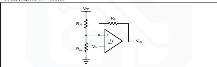
Figure 4. Inverting Comparator with Hysteresis
