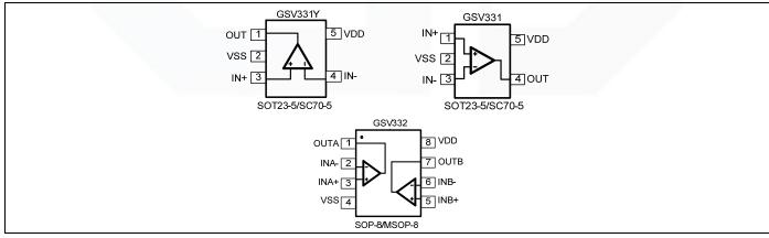
Figure 1. Pin Assignment Diagram
